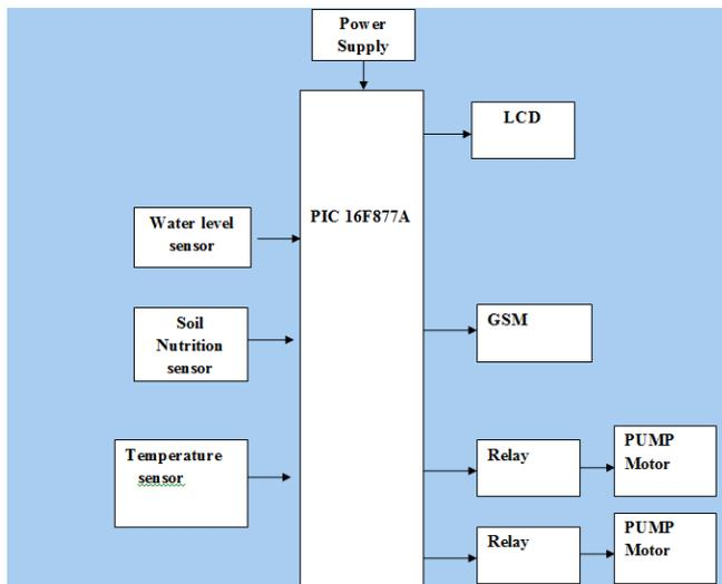
Fig1.Architecture for smart irrigation and nutrition monitoring system
