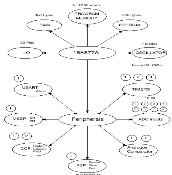
Only 35 single-word instructions is to learn and All single-cycle instructions except for program branches, which are the two-cycle, Operating speed: DC – 20 MHz clock input and DC – 200 ns instruction cycle, Up to 8K x 14 words of the Flash Program Memory, Up to the 368 x 8 bytes of the Data Memory (RAM), Up to 256 x 8 bytes of EEPROM Data Memory, Pinout compatible to the other 28-pin or 40/44-pin PIC16CXXX and PIC16FXXX microcontrollers are used.
