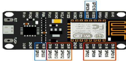
FIG. 3 ESP8266 GPIO Pins
