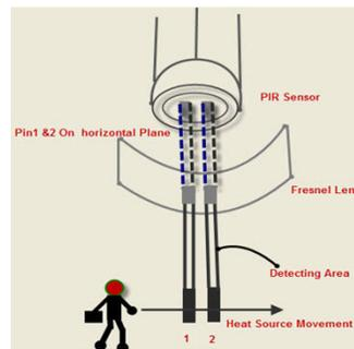
FIG. 6 PIR Sensor function
