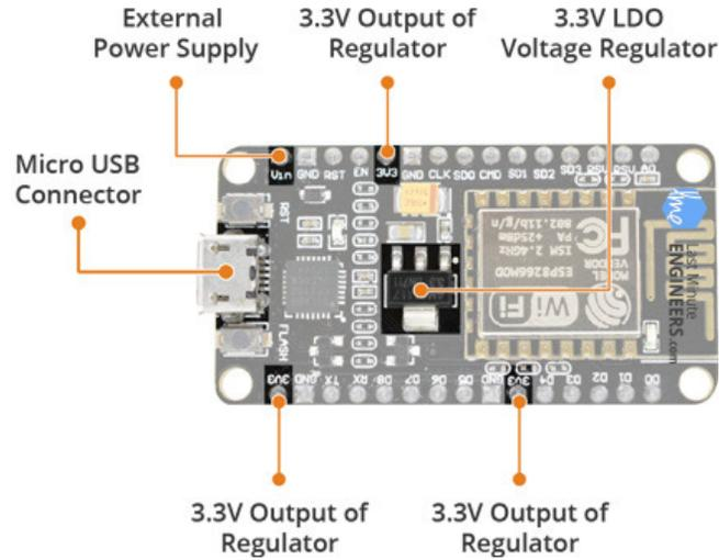
FIG. 4 ESP8266 Power Pins
