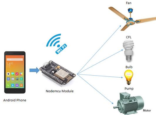
Fig 12. ESP8266 as Access Point
