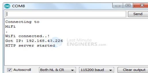
Fig 13. IP address Generation
